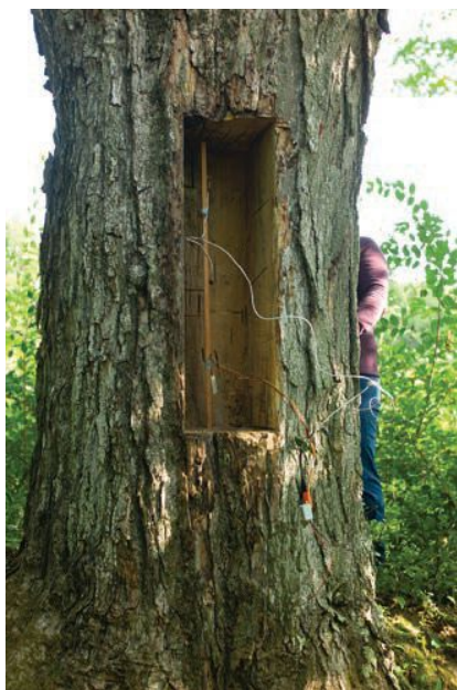
Fig. 2 Views of the cavities inside the maple tree and the wooden box. One sees the temperature sensor in each cavity, positioned 25 inches (64 cm) above the floor.
