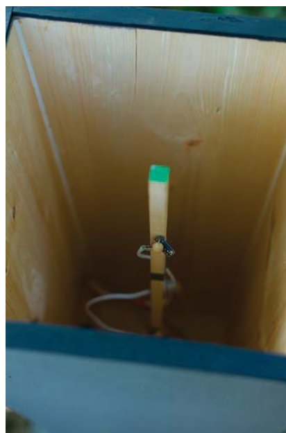
Fig. 2 Views of the cavities inside the maple tree and the wooden box. One sees the temperature sensor in each cavity, positioned 25 inches (64 cm) above the floor.
