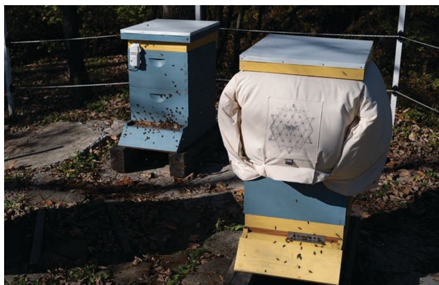
Fig. 6 Setup for measuring temperatures inside occupied Langstroth hives, one without insulation and one protected with a wool hive blanket (Beehive Cozy Cover) that covered the upper, deep hive body. Both hives had a south-facing exposure, an entrance reducer, and a moisture box filled with wood shavings above the upper box (to control condensation). The colonies went into winter with similar bee populations, as estimated by counting the number of full frames of bees.
