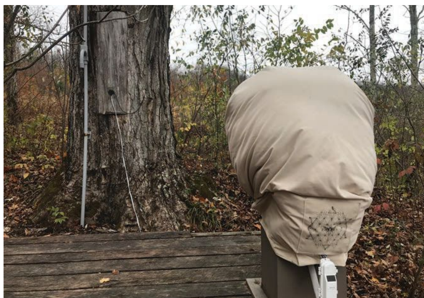
Fig. 3 The completed tree and wooden-box cavities without insulation (left; winter 2019-2020) and with insulation (right; winter 2020-2021). Wires for temperature sensors lead into each entrance.
