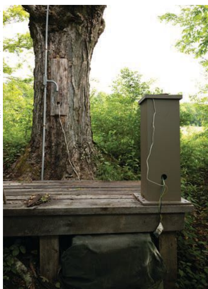
Fig. 3 The completed tree and wooden-box cavities without insulation (left; winter 2019-2020) and with insulation (right; winter 2020-2021). Wires for temperature sensors lead into each entrance.
